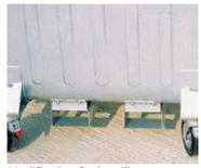
Modification for handling by fork-lift truck.
