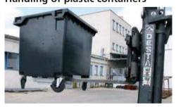
Adapter for handling with a fork lift truck.
