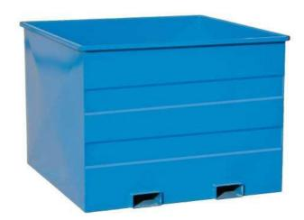
(Ilustrative photograph) 1200 1200 Technical data Steel sheet Material Capacity 1300 I 1144 1144 Weight 121,5 kg 950 Load capacity 500 kg Skid distance 525 mm Pouch dimensions 175 x 80 mm 1200 Width 1200 mm Depth 1200 mm Height 950 mm
